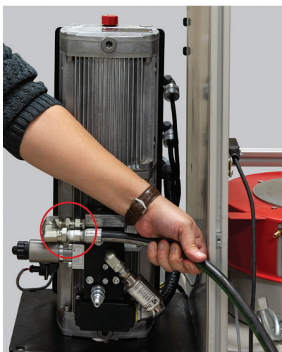
Photo #7— Attach hose to hydraulic line on pump.
