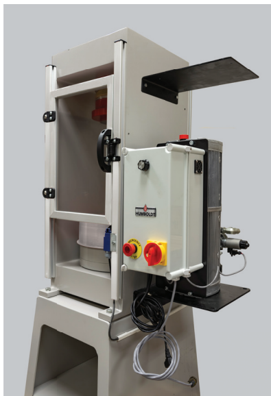
Photo #4— mounting controller bracket
