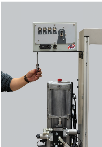
Photo #5— attaching controller to support bracket
