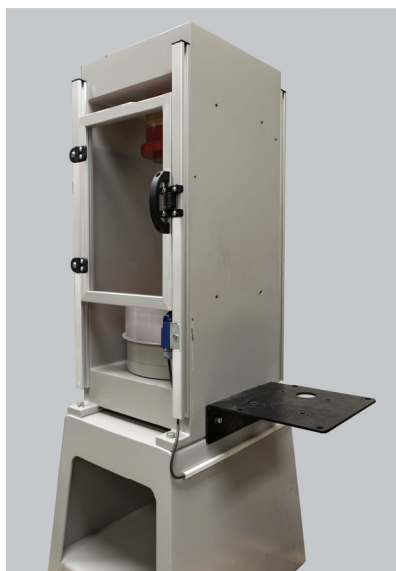
Photo #1— mounting pump support bracket
