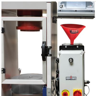
Photo #10— Fill pump with hydraulic oil.
